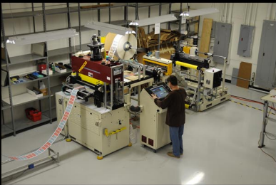
Preco roll die cutting using camera registration ensuring every part is cut accurately within \pm 0.10
