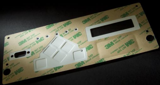
Hand laminating of adhesive for sub-surface printed polycarbonate overlays and nameplates.
