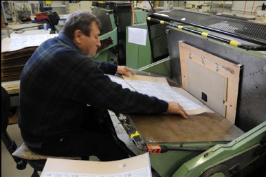
Part pinned on die press for accurate registration on every part.
